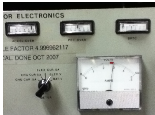
Figure 16 Close up view of the sensor electronics panel meter and control switch.
