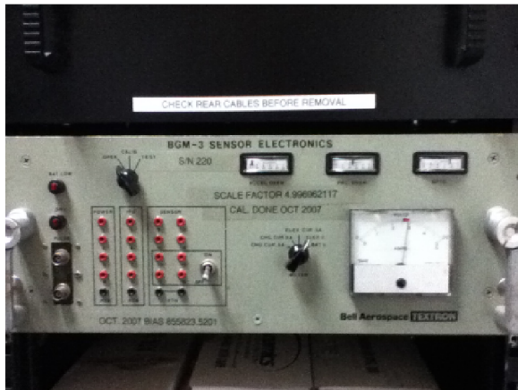
Figure 15: Left: Front of the sensor electronics case. The sensor test points are on the left side of the case. The panel meter is on the right side. Right: Close up of the left side of sensor electronics drawer. When receiving a sensor, always check the battery low light before plugging in the sensor. If it is lit, notify pfpe-internal@whoi.edu immediately.
