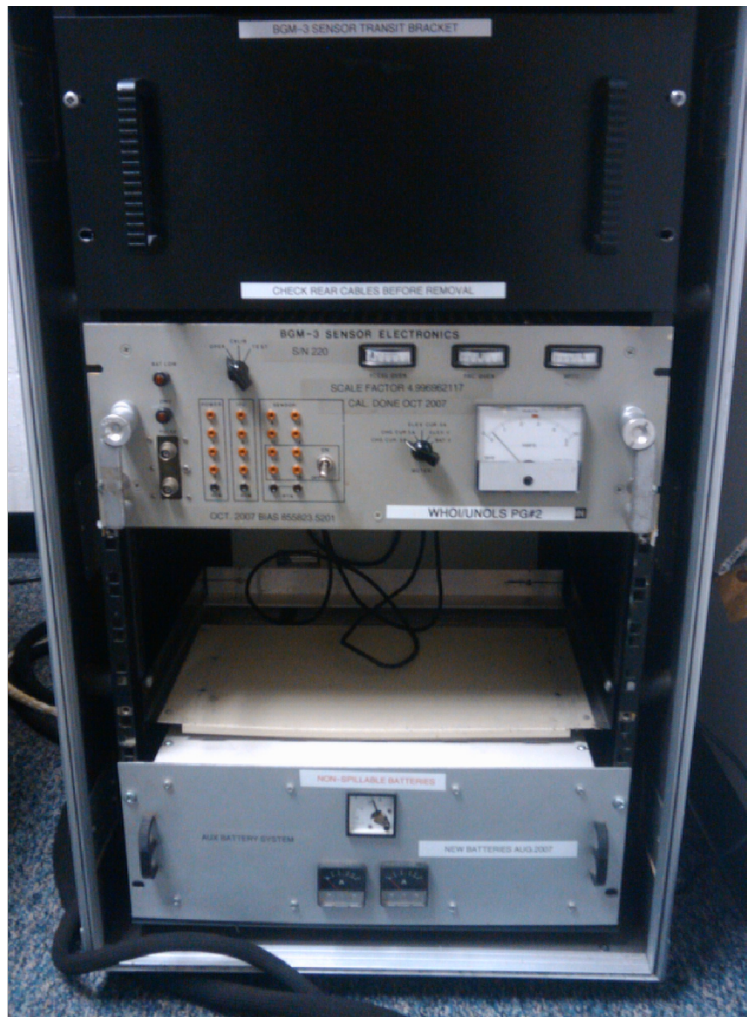
Figure 14: The BGM-3 sensor in its shipping case. The auxiliary battery is at the bottom of the case; the primary sensor battery above it (in the rear); and the sensor electronics above it. The sensor is in the shipping bracket behind the black panel at the top of the case.
