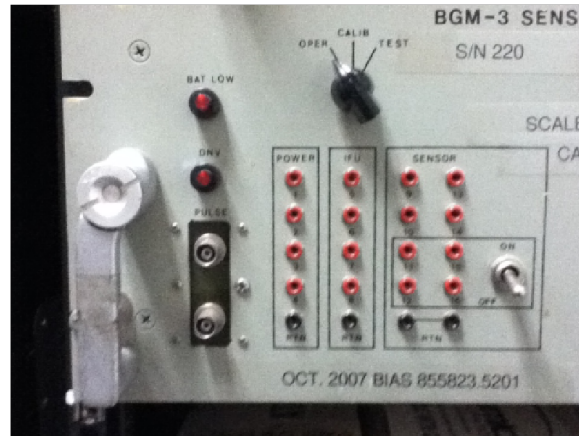
Figure 15: Left: Front of the sensor electronics case. The sensor test points are on the left side of the case. The panel meter is on the right side. Right: Close up of the left side of sensor electronics drawer. When receiving a sensor, always check the battery low light before plugging in the sensor. If it is lit, notify pfpe-internal@whoi.edu immediately.
