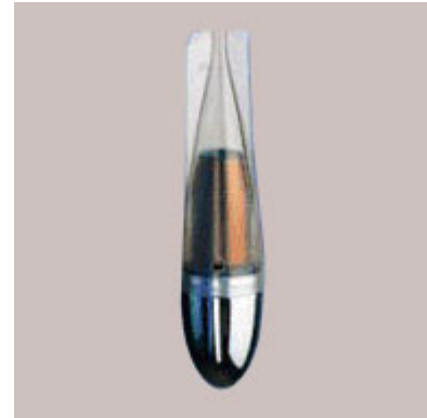
FIGURE 1-3: XBT Probe
