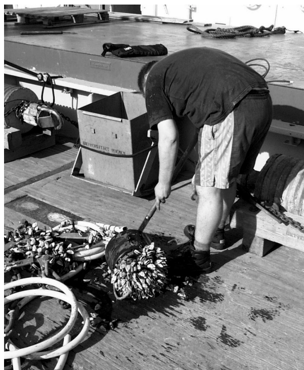
Fig. 15: Intense biofouling at the remote transducer head and at the 25 m chain of the DOME surface buoy.
