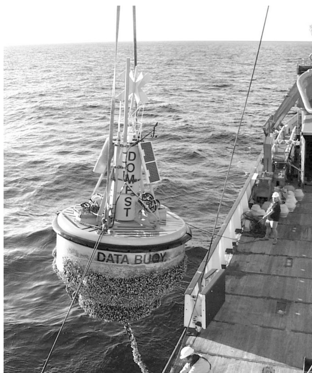
Fig. 14: DOME surface buoy during recovery. Visible is the intense biofouling on the subsurface of the buoys hull.
