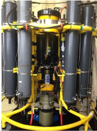
Photo 1: Instruments and battery pack on rosette. UVP is not mounted in this photo.
