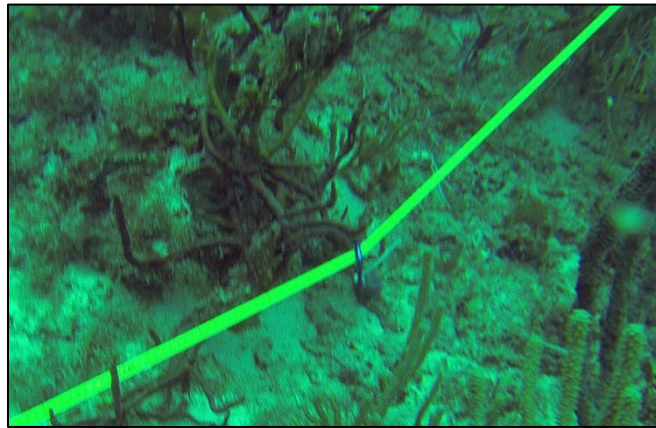
Figure 1. Example of weight attached to transect tape.
