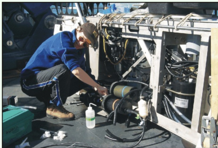
Figure 22. New mounting system for the ac-9s on BIOMAPER II. Anne Canaday conducting a pure water calibration of the ac-9s. The Hydroscat-6 is visible in the aft bay.
