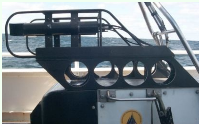
Figure 16. The extension bracket used to elevate and move the VPR forward.
