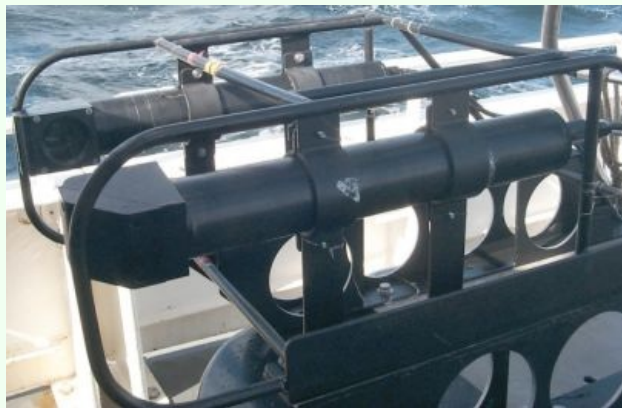
Figure 15. The single camera VPR on BIOMAPER II. Strobe is in the canister in the background and camera is in the foreground.
