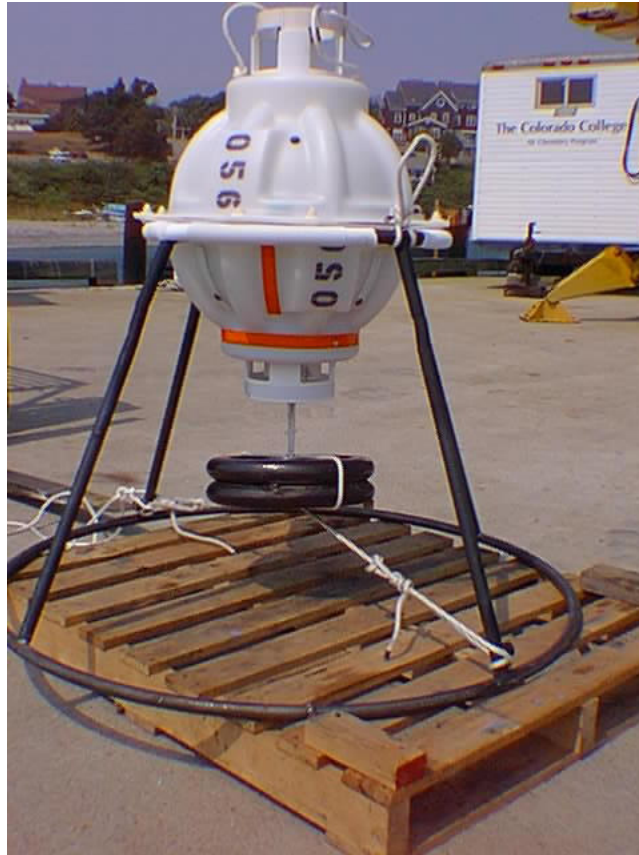
Photo 12-1 Anchor/Platform Attachment to C-PIES
