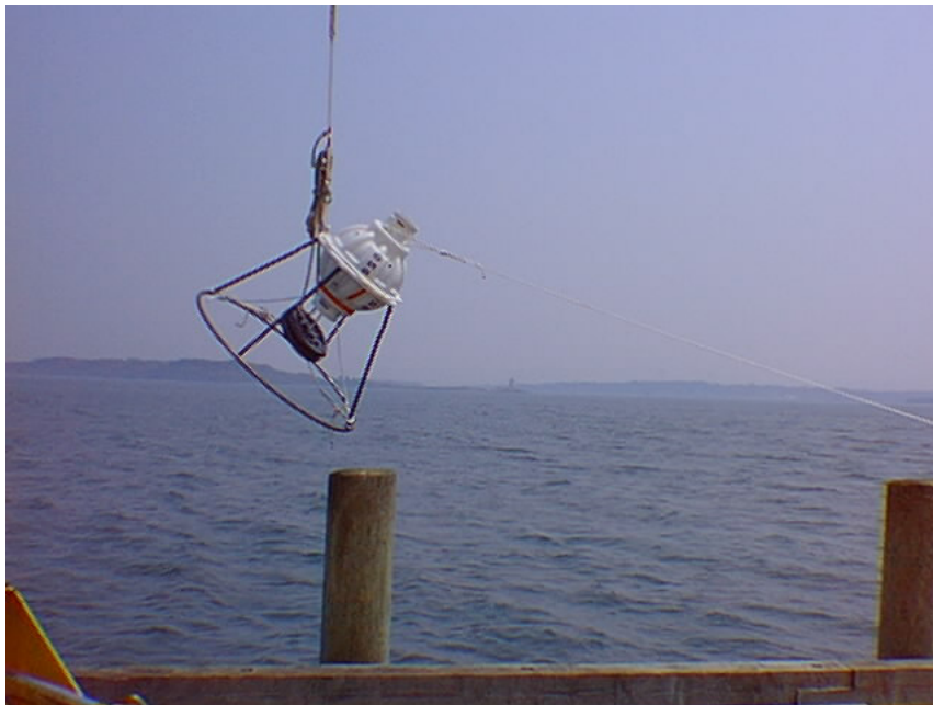
Photo 12-2 Lifting Point for C-PIES Deployment
