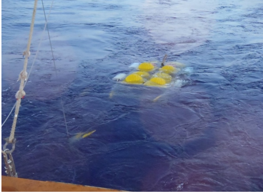
Fig. 2. Injection sled just after deployment. The sled is slightly buoyant at the surface due to the glass balls and the compressible white fenders. The sled is streaming behind the wire with the ship underway at about a knot. The yellow boots at the forward end of the sled bridle can be seen below the water surface where they are attached to the end of the CTD cable via a pear-ring. Suspended from the pear-ring is a 50-meter cable with an 850-pound hydroweight at the bottom. The sled becomes less buoyant as it descends because the fenders compress. They expand again upon surfacing to facilitate recovery.
