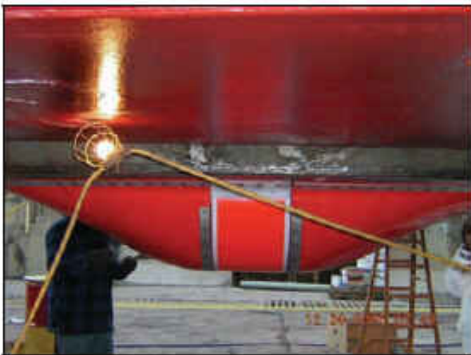
Fig 1: EM1002 transducer fairing
