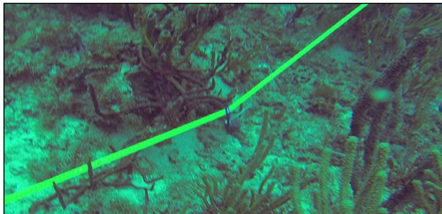
Figure 3. Example of weight attached to transect tape.
