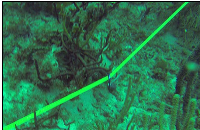
Figure 1. Example of weight attached to transect tape.
