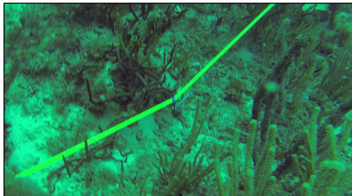
Figure 2. Example of weight attached to transect tape.
