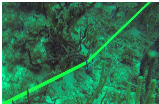
Figure 1. Example of weight attached to transect tape.
