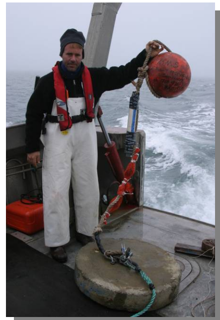
Mussel mooring w/acoustic pinger
