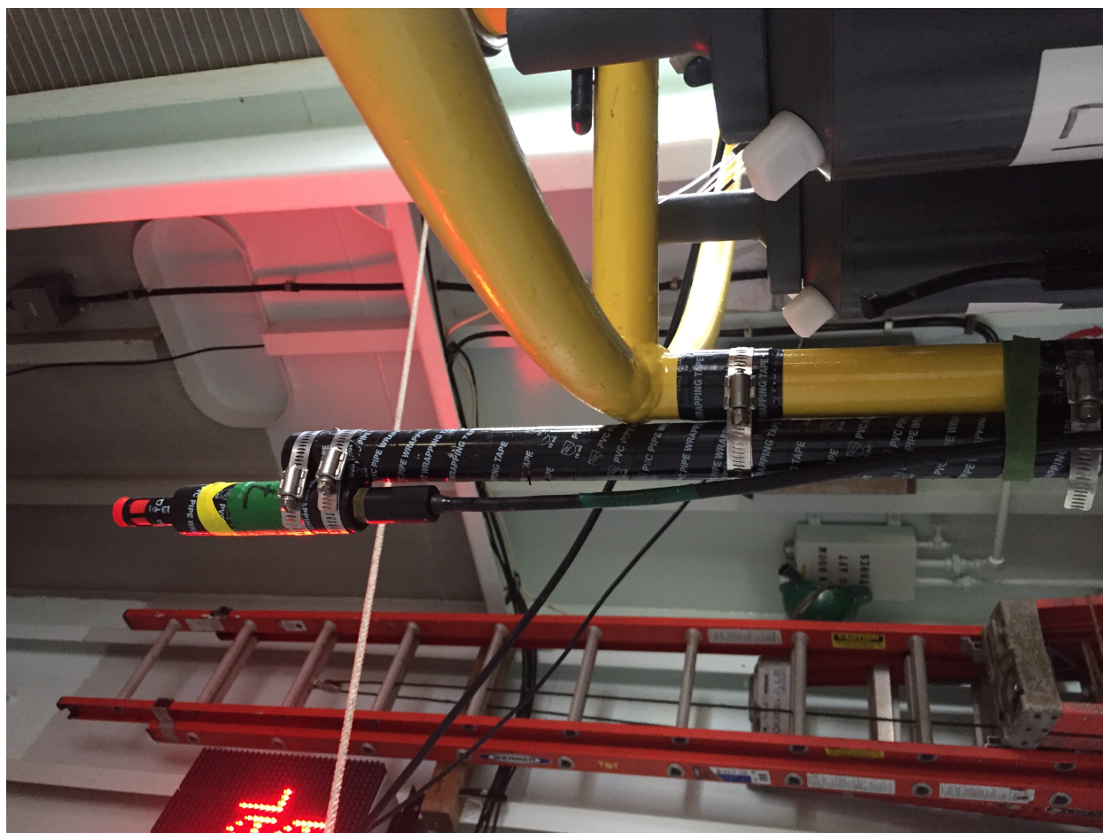
Fig. 1: Upward-looking chipod sensor attached to the rosette
