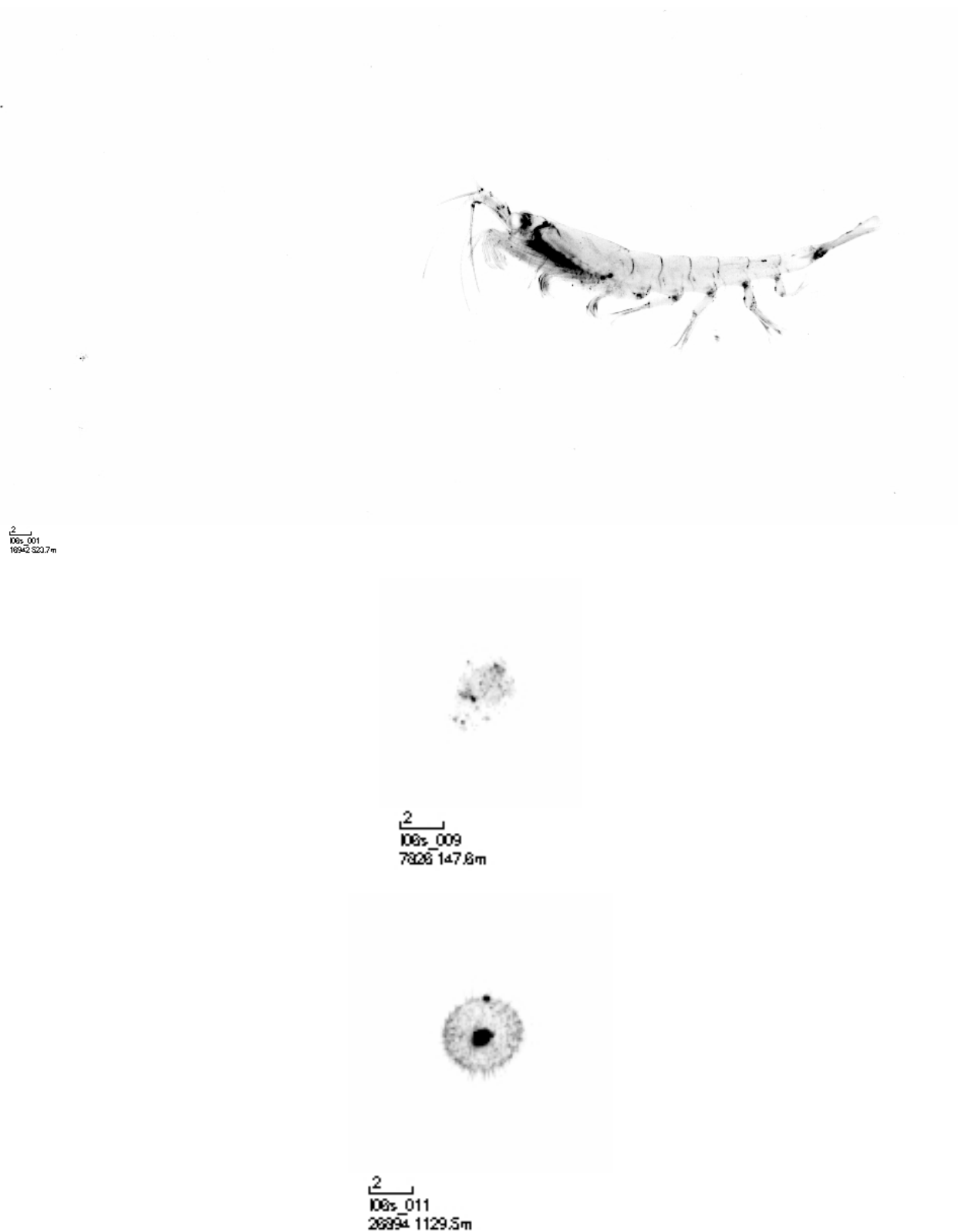
Fig. 2: Figures 2 to 11 - Examples of particle and plankton images captured by the UVP5HD and processed by custom software. The scale bar indicates 2 millimeters. Station number, image number for that cast, and depth at which the image was captured are also given in the image.
