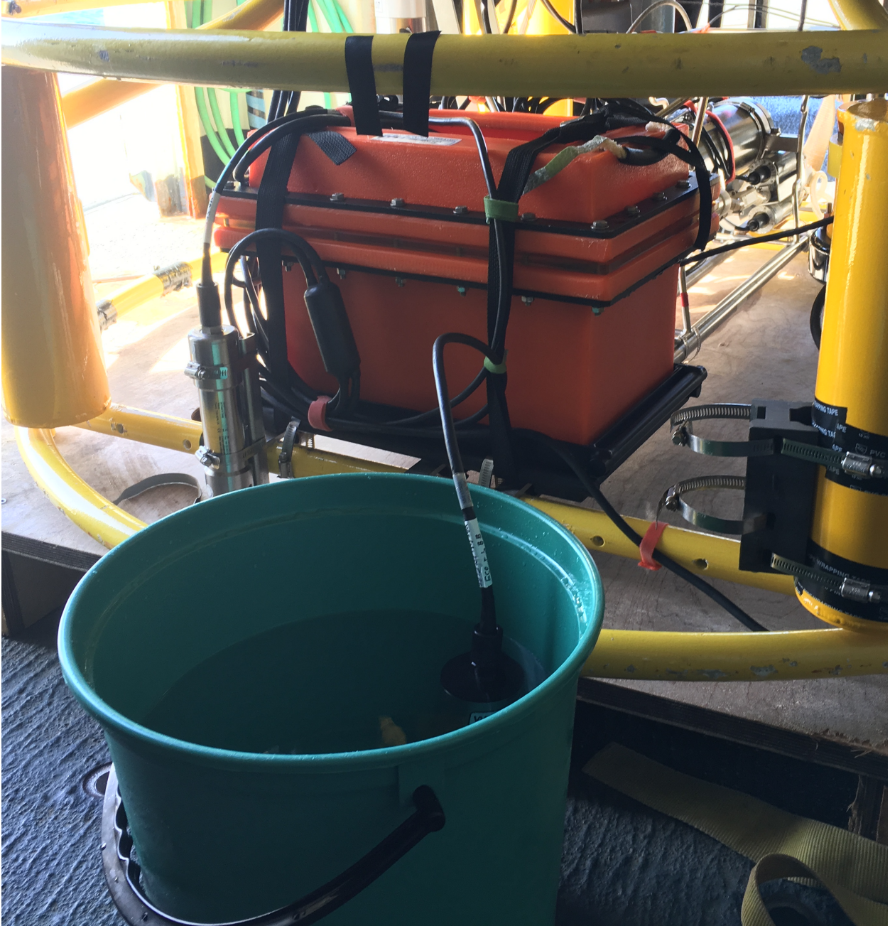
Fig. 8: FLBB readings taken on deck post last station. FL average reading was 0.050 volts, BB average reading was 0.070 volts.
