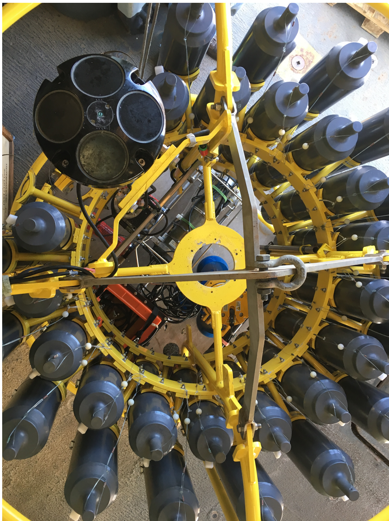
Fig. 2: Package sensor setup with top as southeast, to show in order from top clockwise CTD, downward LADCP, LADCP battery, and UVP.
