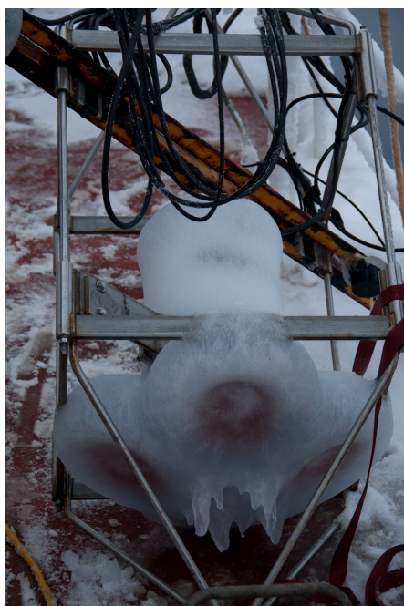
Figure 11. Ice accumulated on the ADCP during the cruise (Photo by Jeffrey Charters).
