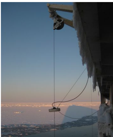
Figure 8. The ‘de-icer’ attached to the CTD wire.
