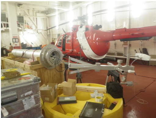
Figure 2: Assembled mast minus the scan head for the UV/Vis spectrometer and wind sensor.
