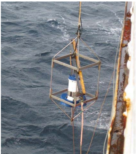
Figure 2. ADCP being lowered to 5m during rosette cast. Photo by Sarah Zimmermann
