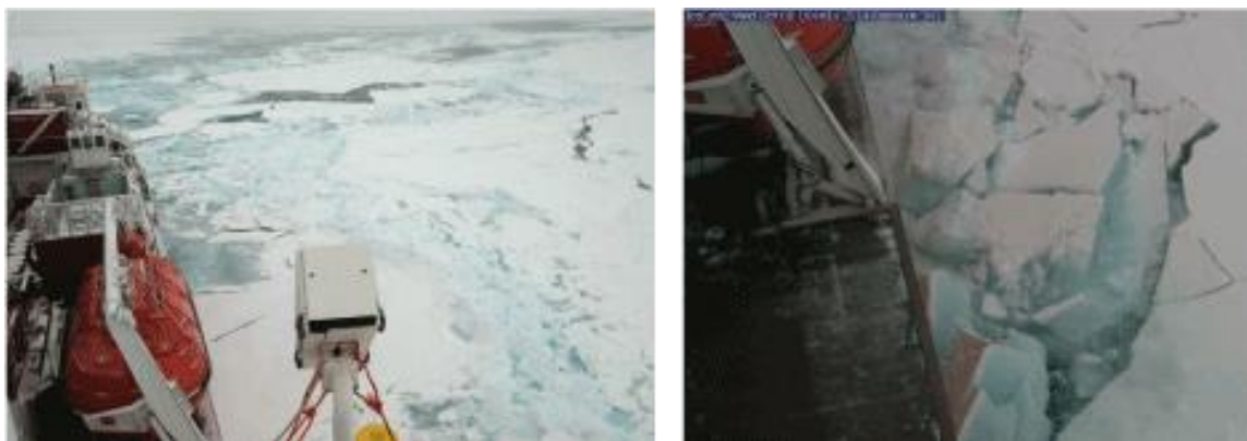
Figure 3: (left) Downward facing NetCam on the port side of the ship. (right) Example image from the NetCam showing the measuring stick (the colors indicate 10/50 cm intervals) which is often used to estimate ice thickness
