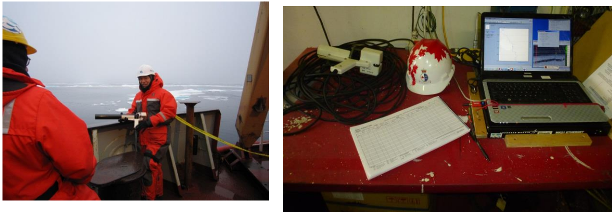
Figure 1: XCTD probe deployment from the ship's stern (2011) and XCTD setup showing launcher, log book, and laptop sitting on top of data converter Win MK-21.
