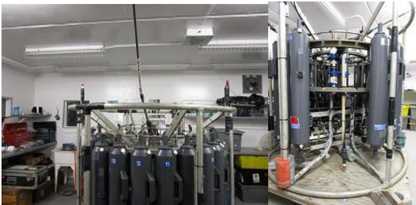
Figure 2 Chipods mounted on the rosette.
