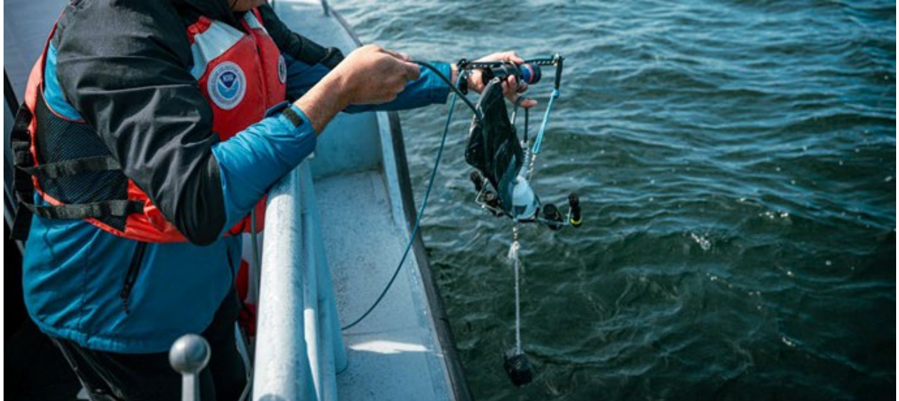
Figure 6. The camera operator deploys the camera with the accessories and USBL transponder (Nano) attached. Photo: Kaden Staley (MTU)
