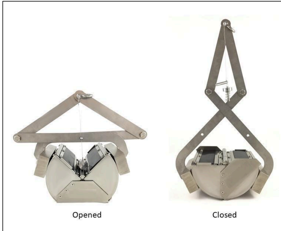
Figure 1. Standard Ponar Sample in the opened and closed positions, Photo modified from Aquatic BioTechnology, Inc.
