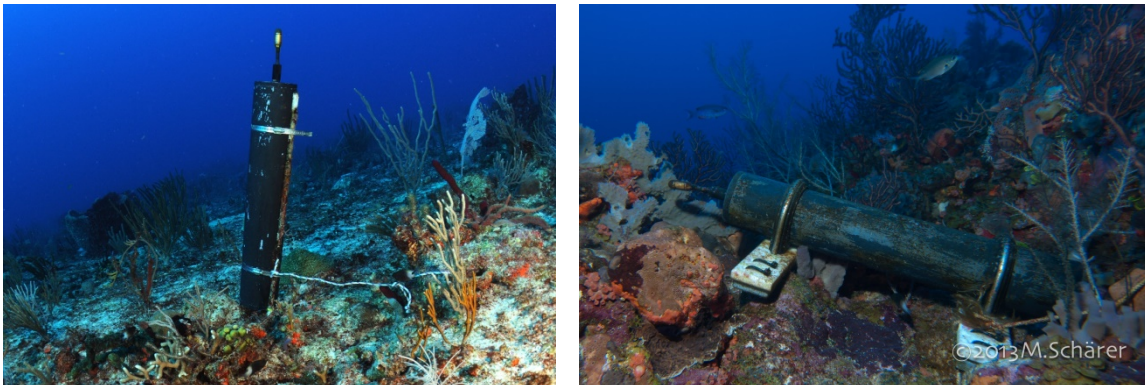
Figure 2. Deployment methods for DSGs on the seafloor, vertical rebar attachment at left (photo by J. Zegarra), horizontal weighted base attachment at right (photo by M. Schärer).
