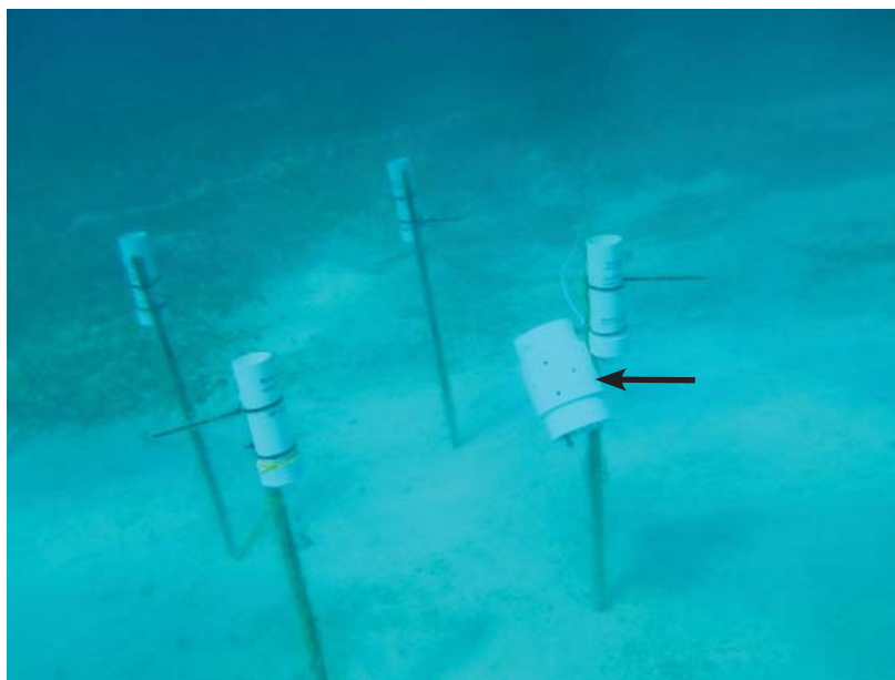
Figure 6.4. POCIS deployment canister (arrow) among the sediment traps at a site in the STEER.
