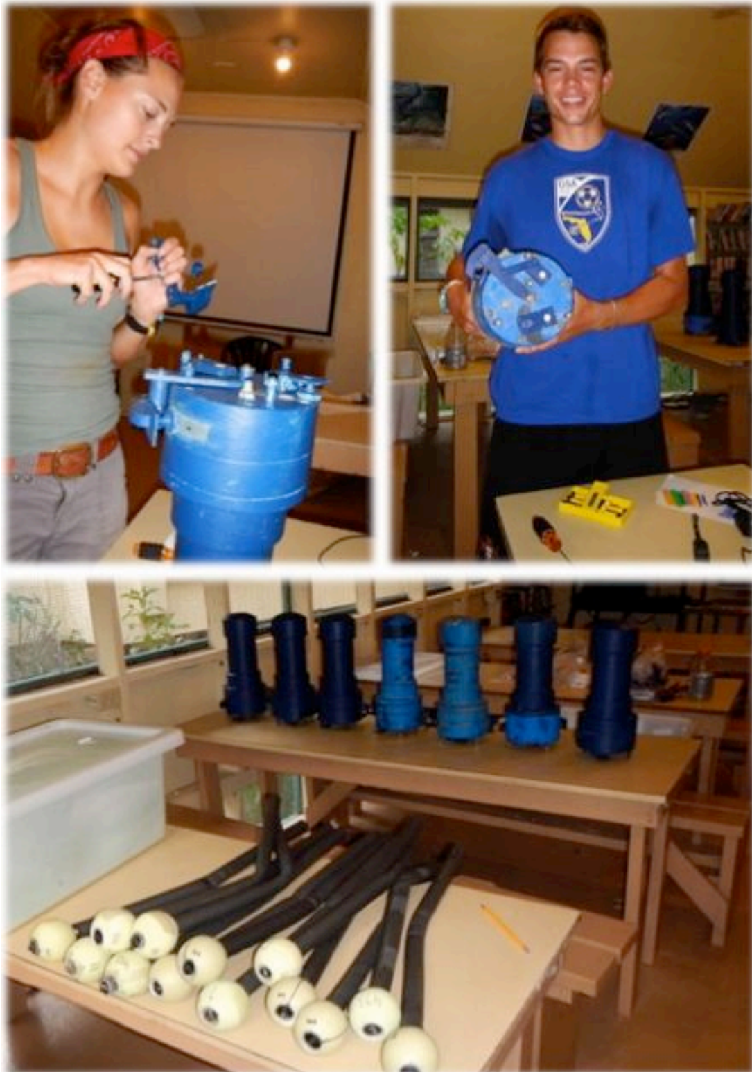
Figure 3. Before the nephelometers (blue cylinders above) could be deployed, they had to be repaired and tested. Marrotte current meters (or “lollypop”) shown with yellow bulbs on the table below also needed to be tested.
