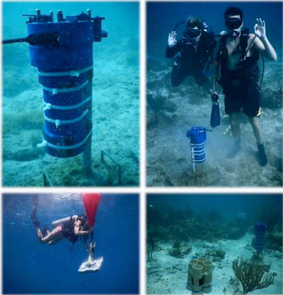
Figure 4. Concrete base housings were taken to the seafloor and then nephelometers attached using zip ties. The nephelometers and Marrotte current meters were deployed within 5 meters of the sediment traps (below right).
