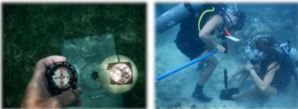
Figure 5. The Marrotte current meters were deployed on fence posts or concrete footings (left) or hammered into the sea floor (right). Their bulbs need to be oriented such that the black line is north.
