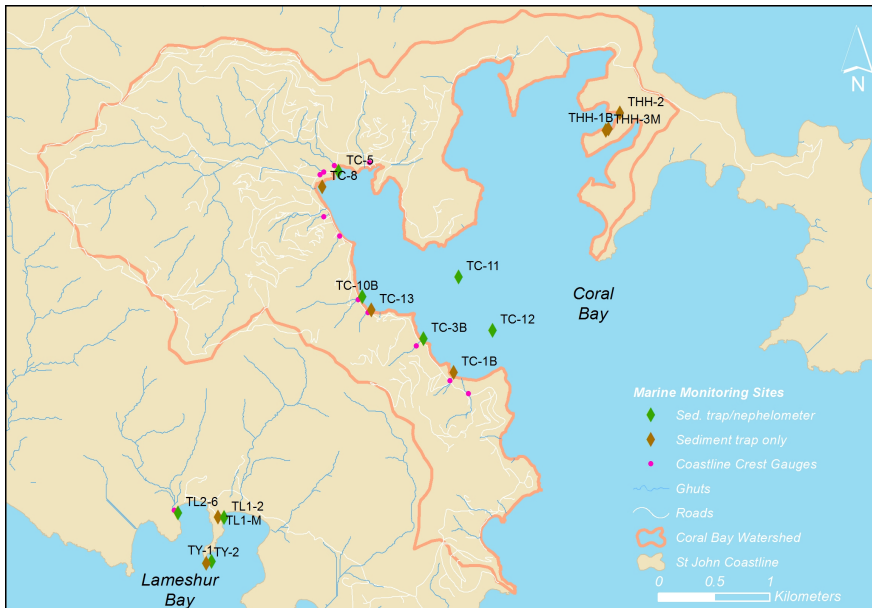
Figure 2. Map showing the marine monitoring locations (diamonds) with sediment traps and corresponding coastal crest gauges (pink dots). Instrument packages (nephelometer and 2 Marotte current meters) are deployed adjacent to the sediment traps and are located at 8 sites (marked by green diamonds).
