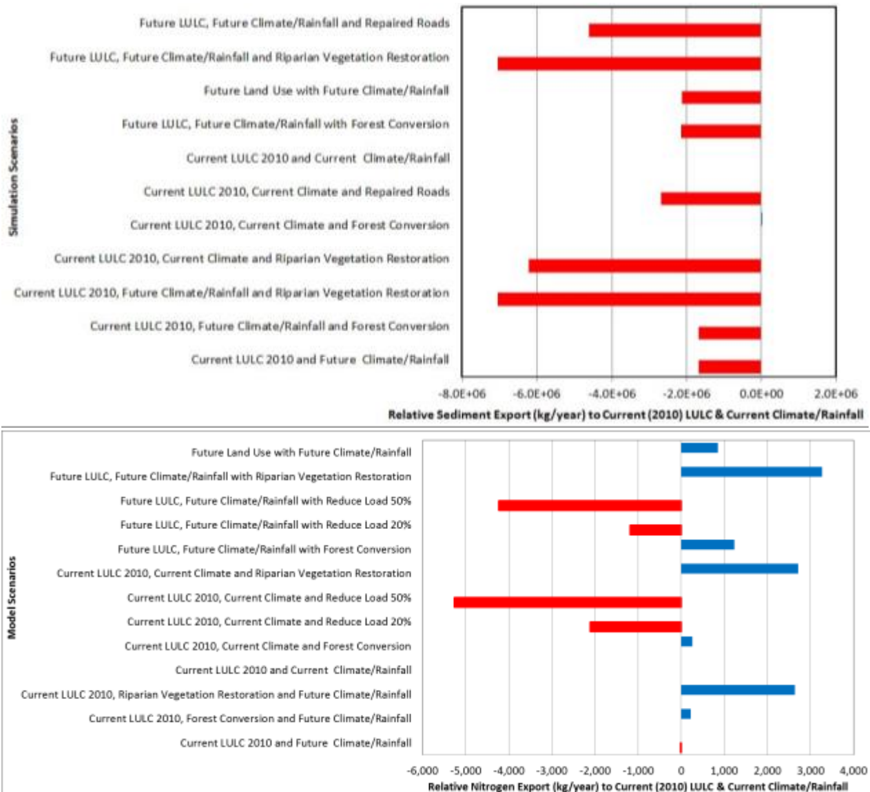
FIGURE 12. COMPARISON OF RELATIVE A. SEDIMENT EXPORT B. NITROGEN EXPORT FOR ALL THE MODELLED SCENARIOS FROM 2010 LULC & CURRENT RAINFALL.
