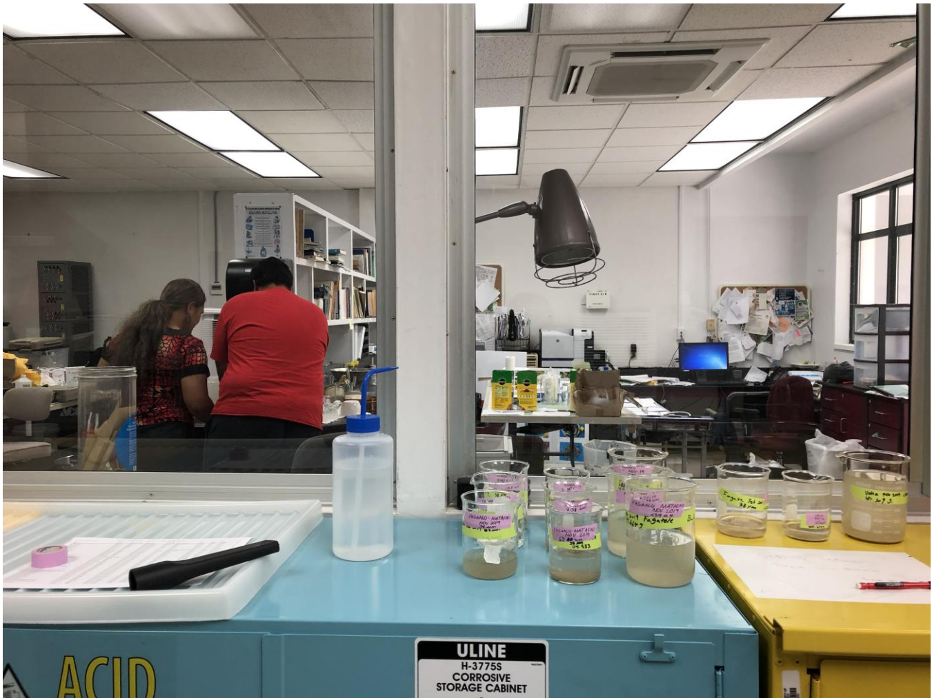
Figure 7. ASCC Marine Science students Warren Sevaaetasi and Perosi Vaofanua processing sediment samples in the Natural Resource laboratory with salt-removed sediment samples (foreground) allowed to settle for 24-48 hours prior to drying in the oven.
