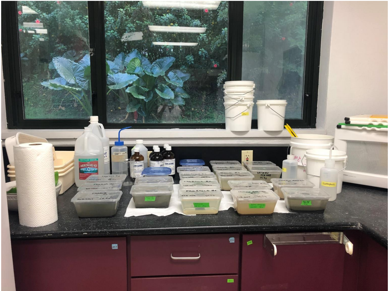
Figure 6. Sediment salt removal process. Wet sediment samples from each sediment trap were transferred to individual 1 L plastic containers, and left for 24-48 hours to allow sediment particles to settle.
