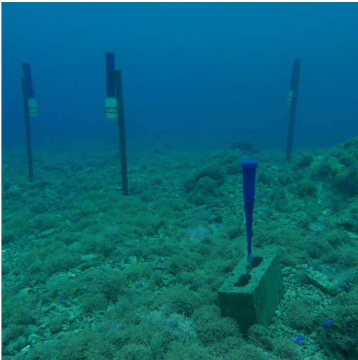
Figure 3. Three SediSampler ® patented traps (Integral Aqua Pty Ltd) on the reef slope at each site in 5-7 m depth. Each trap was attached to a steel bar driven into the substratum so that the mouth of the trap was positioned approximately 1 m above the substratum
