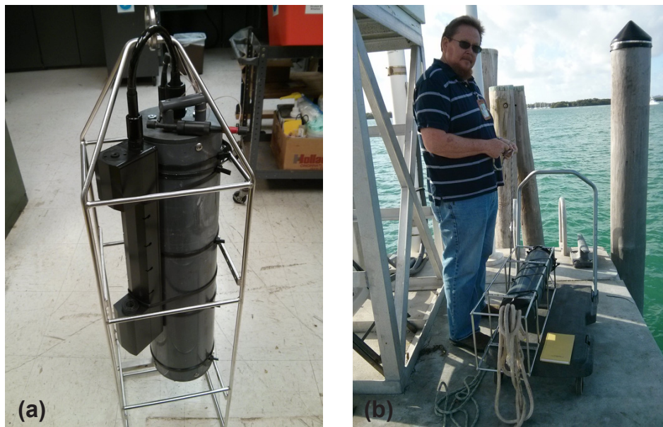
Figure 8. (a) WETLabs C-STAR sensor housed in a deployment cage; (b) WETLabs C-STAR sensor ready for deployment.
