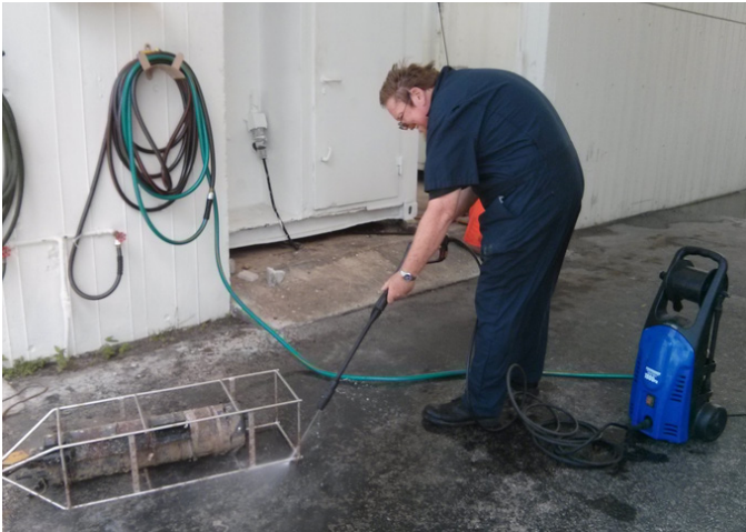
Figure 9. WETLabs C-STAR sensor undergoes extensive cleaning after deployment due to environmental fouling.
