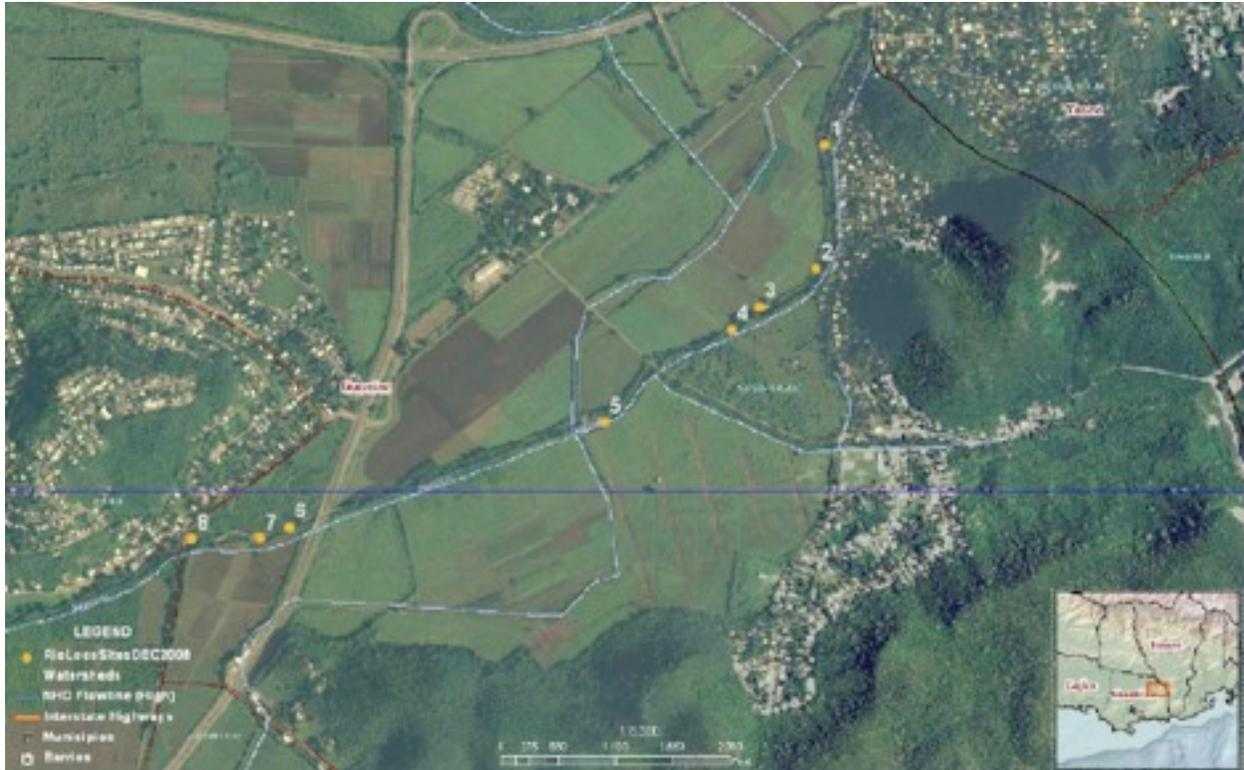
**Figure 1. Shows the primary locations of severe erosion in the Rio Loco as is summarized in our field technical memo (Sites 5 and 6 are the two locations where instream structures are still contributing to river channel erosion)**
