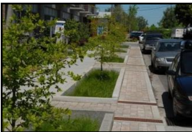
Figure 12. Rain garden from St. Croix and streetscape biofilters from Santa Monica, CA
