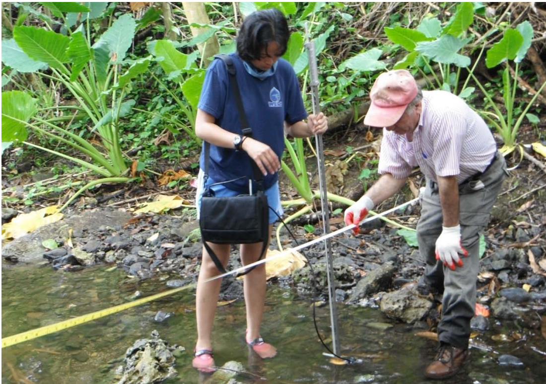
Figure 17: Stream Flow Measurement in Masso River (March 12, 2012)
