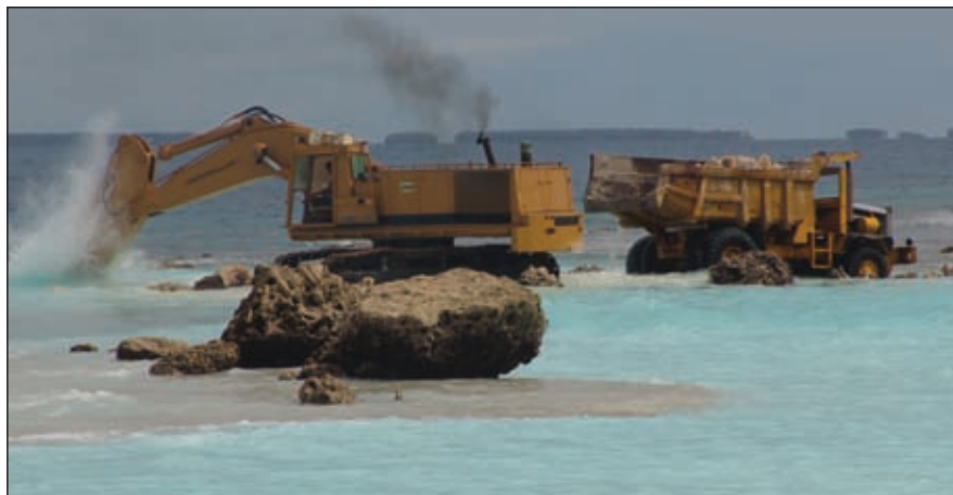
Figure 12.8. Mining of hard rock along edge of lagoon fringing reef near Majuro airport, 2007. Photo: D. Jacobson.
