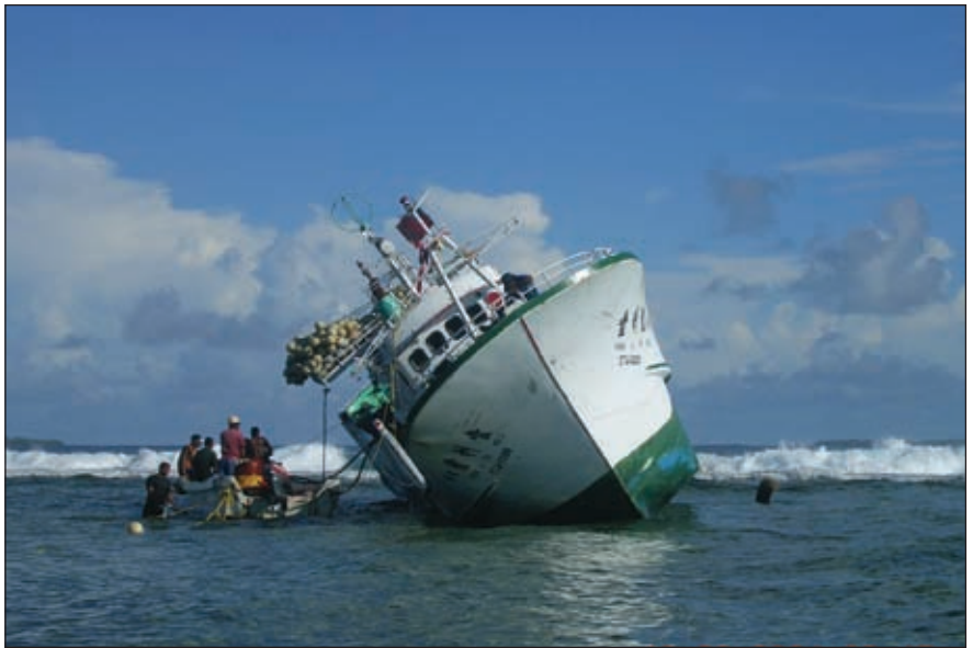
Figure 13.10. Removing oil from a grounded vessel on Elato Atoll in Yap. Photo: L. Johnson.
