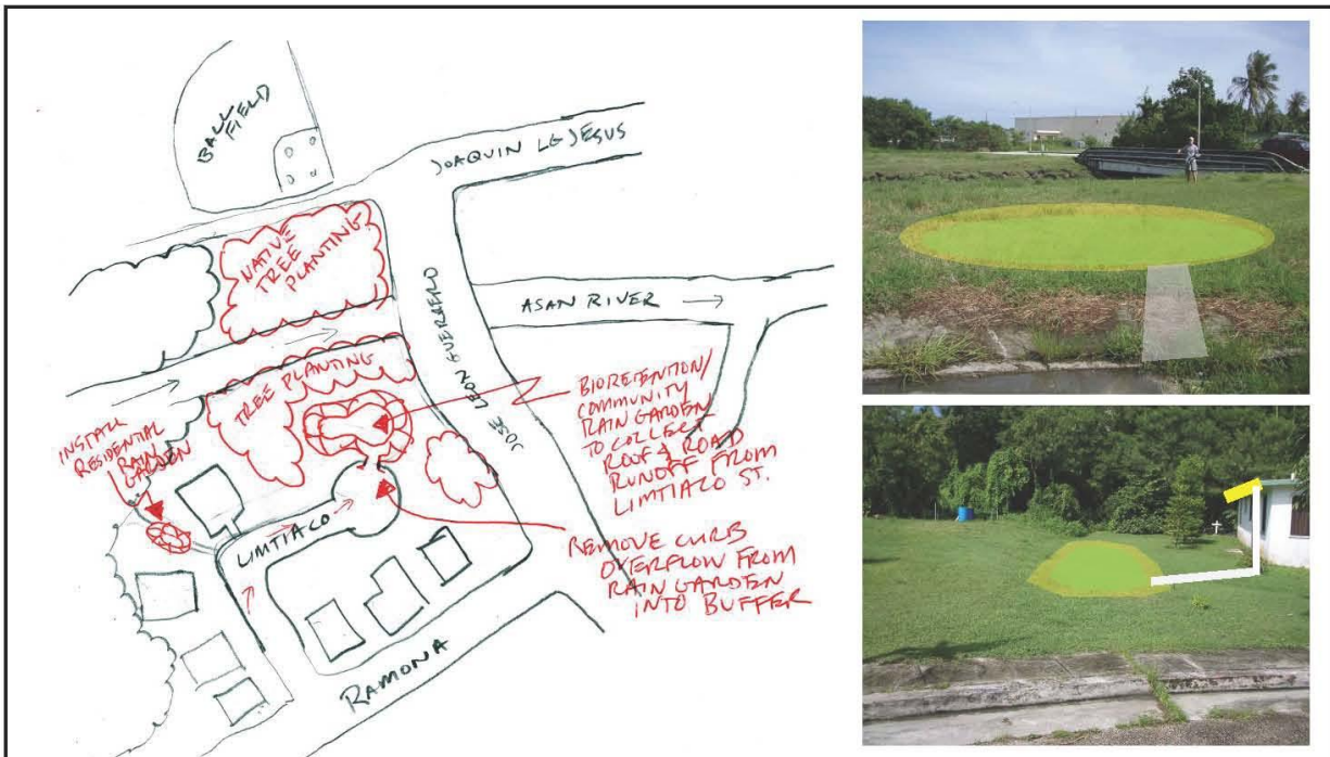
Figure D-17. Plan view of proposed bioretention/community rain garden (conceptual – not to scale) adjacent to the cul-de-sac (top photo) and small rain garden at house up the hill (bottom photo).
