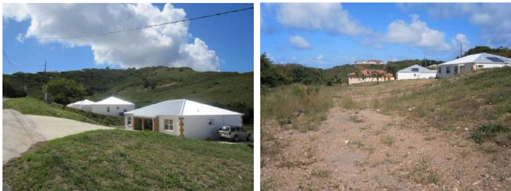
Figure 4.7. New homes were built in the gut upstream from the Seven Flags Rd. erosion (left). The areas behind the houses should be retrofitted to create a series of terraced depressions to help provide more storage and decrease velocities (right).
