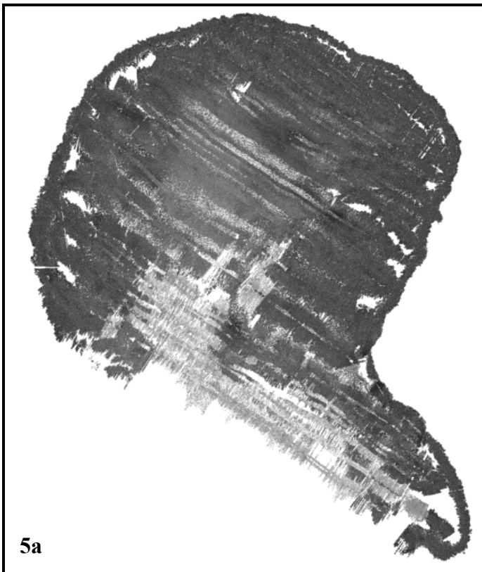
Figure 5: Georeferenced Backscatter. Backscatter was recorded during a multibeam mapping survey in (5a) Fagatele Bay National Marine Sanctuary and at (5b) Taema Bank (Western) in April and May 2001. Light areas are sites of high acoustic return and dark areas are sites of low acoustic return.
