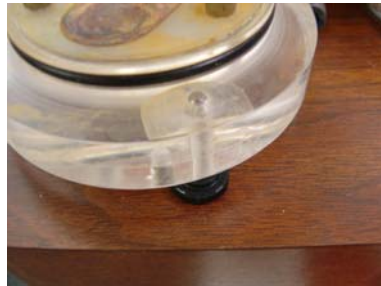
Figure 45. Photo of failed SVS. The housing material around the hold down screw parted during deployment flooding the housing.
