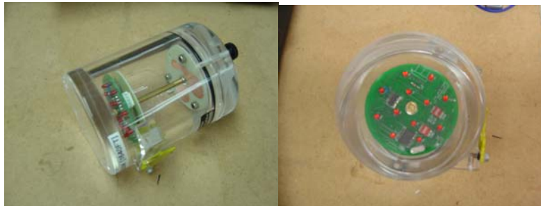
Figure 27. SVS. Left image is an isometric view of the housing. Right image shows the face of the SVS with the diode pattern. The SVS is mounted on the bait arm in such a way as to allow these diodes to be seen in both cameras. The diodes are programmed to fire at a frequency of 30 hz to match the video frame rate on a regular interval.
