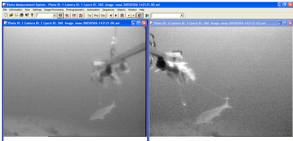
Figure 42. Frame grab of video imported into VMS software. The left image was collected using the ROS Navigator camera, the right image using the Watec camera.
