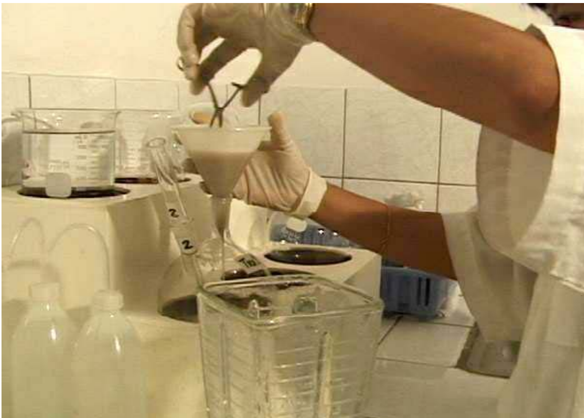
Figure 7. Blended fish tissue being added to the distillation flask using a funnel.
