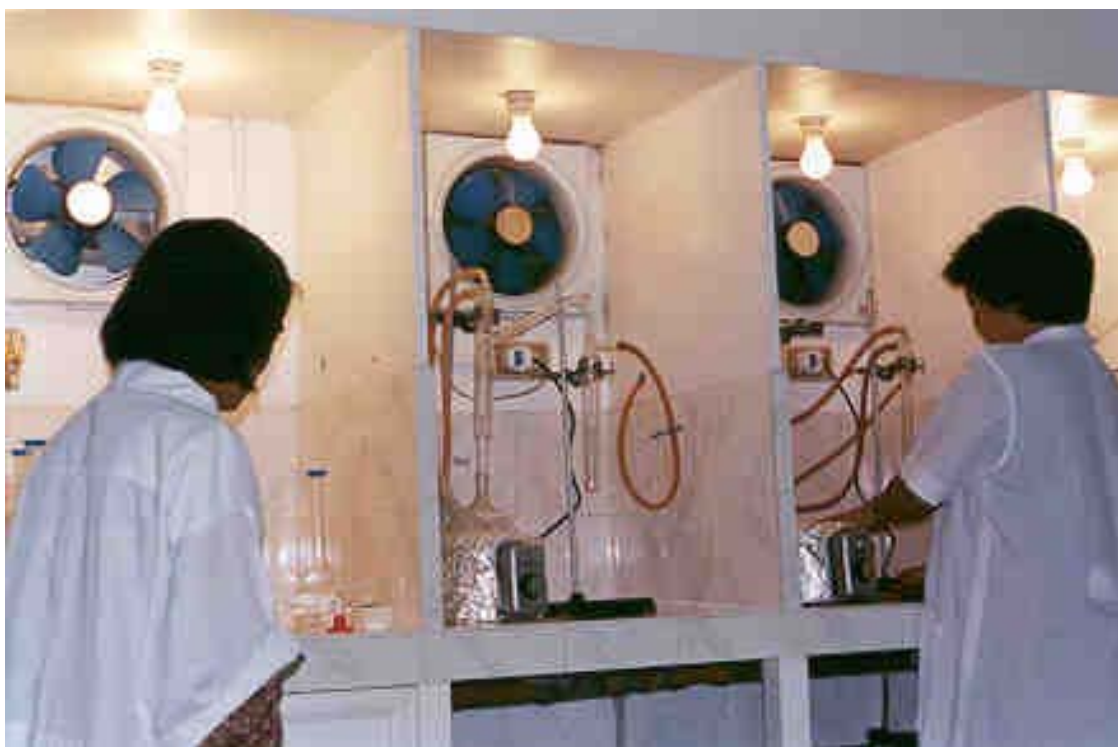
Figure 8. Reflux apparatus being used to digest fish tissues using sulfuric acid to release HCN vapor, which is then captured in the absorber tube containing sodium hydroxide.
