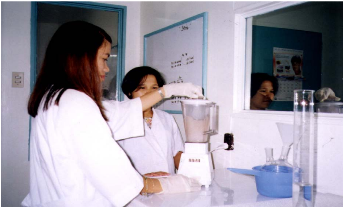
Figure 6. Blending approximately 10 grams of whole fish or internal organs of larger fish in sodium hydroxide solution.
