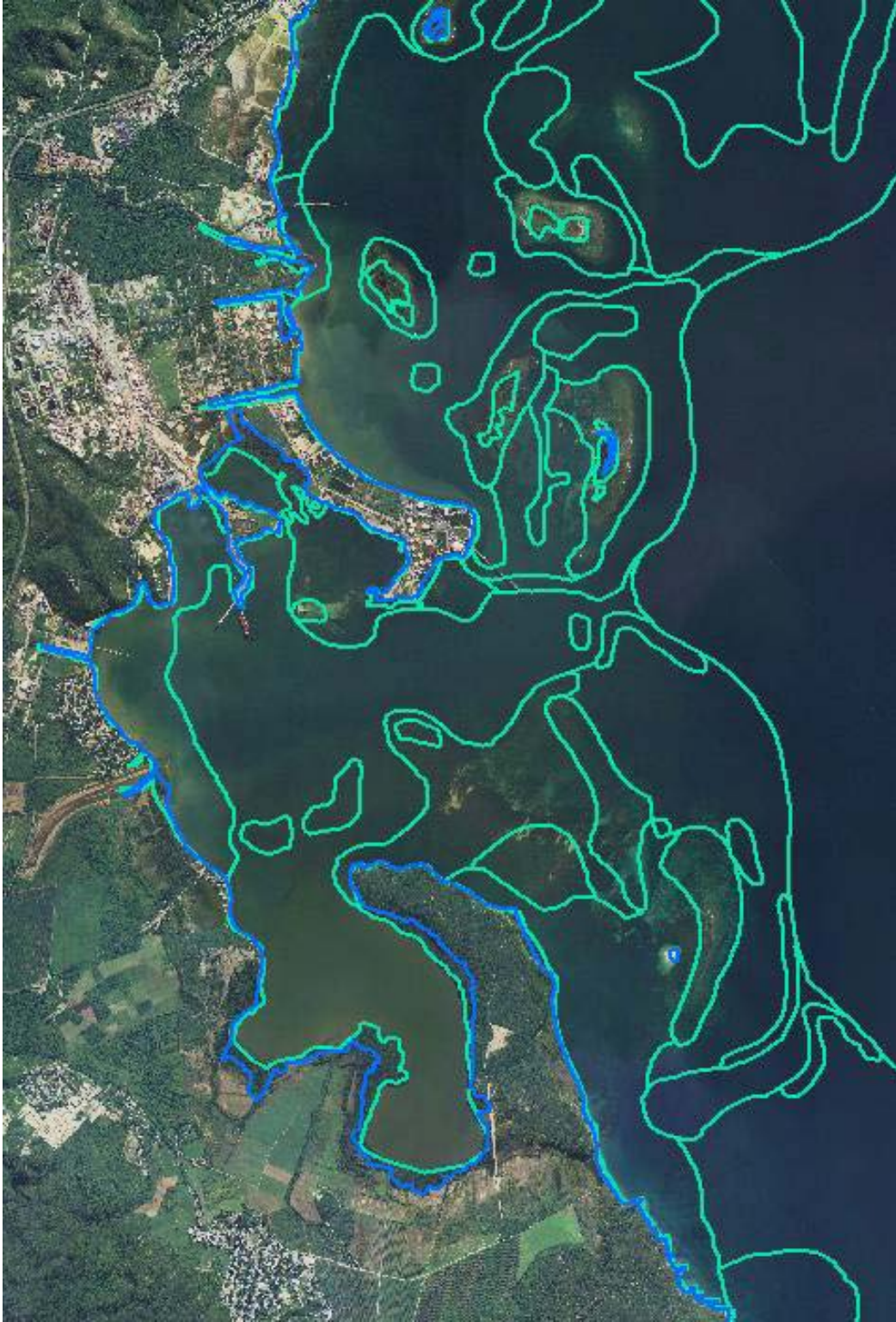
Figure 7. Shifted (in green) shoreline feature from the georeferenced image of map I-2263 overlaid on satellite imagery. The blue line represents the shoreline feature from NOAA benthic habitat map (Kendall et al., 2001). Green line depicts the shoreline along the seaward edge of mangrove habitat whereas the blue line depicts the shoreline along the landward edge of mangrove habitats. Map scale = 1:40,000.
