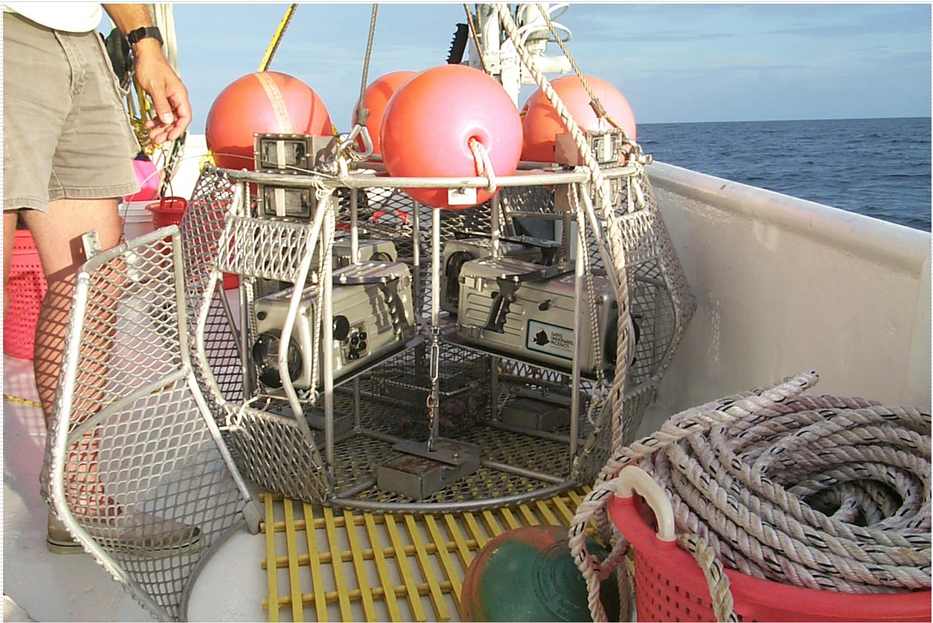
Five camera array using 4 Sony VX1000 digital camcorders in Gates housings, and a single, down-looking Sony PC110 or PC120 digital camcorder in a Gates housing
