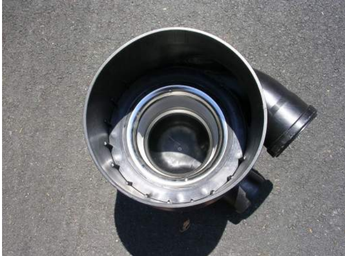
Figure S4.6. Interior of Vortex Filter
