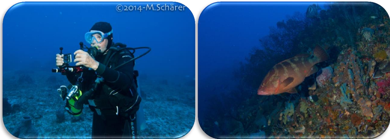
Figure (Left): Video and laser caliper method at left (photo by M. Schärer)
