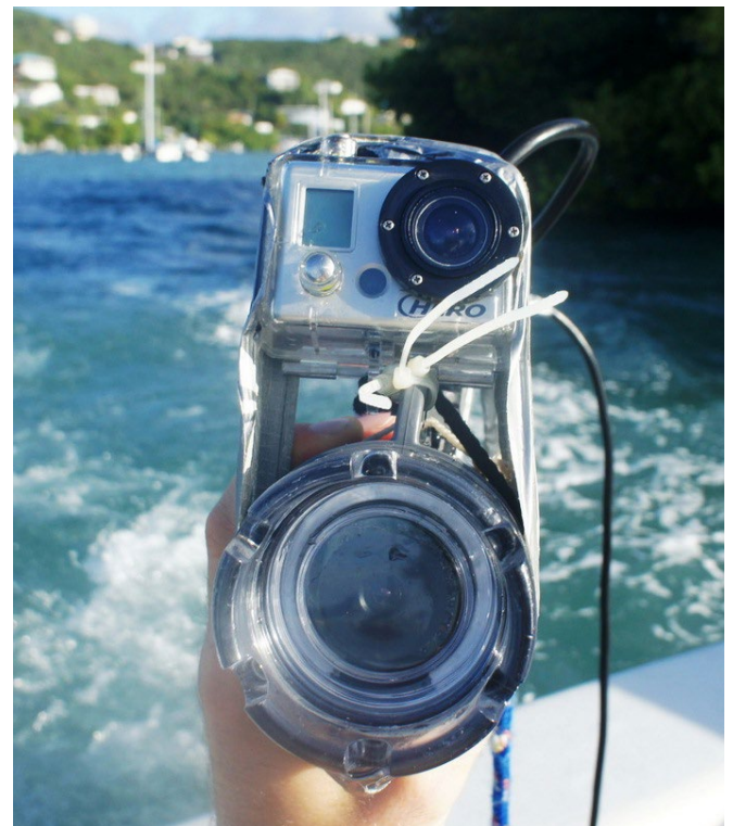
Figure 3.9. We also collected underwater video at several sites using a GoPro camera to compare its video quality with that of the SeaViewer camera. We also used the GoPro video to classify sites that had poor quality SeaViewer video.
