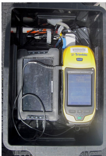
Figure 3.7. Topside field equipment used to collect georeferenced underwater video at GV drop camera sites. While the SeaViewer unit was in the water, we recorded the location of the camera using a Trimble GeoXH GPS receiver (right) while viewing and classifying real-time video footage on a Sea-DVR (left).
