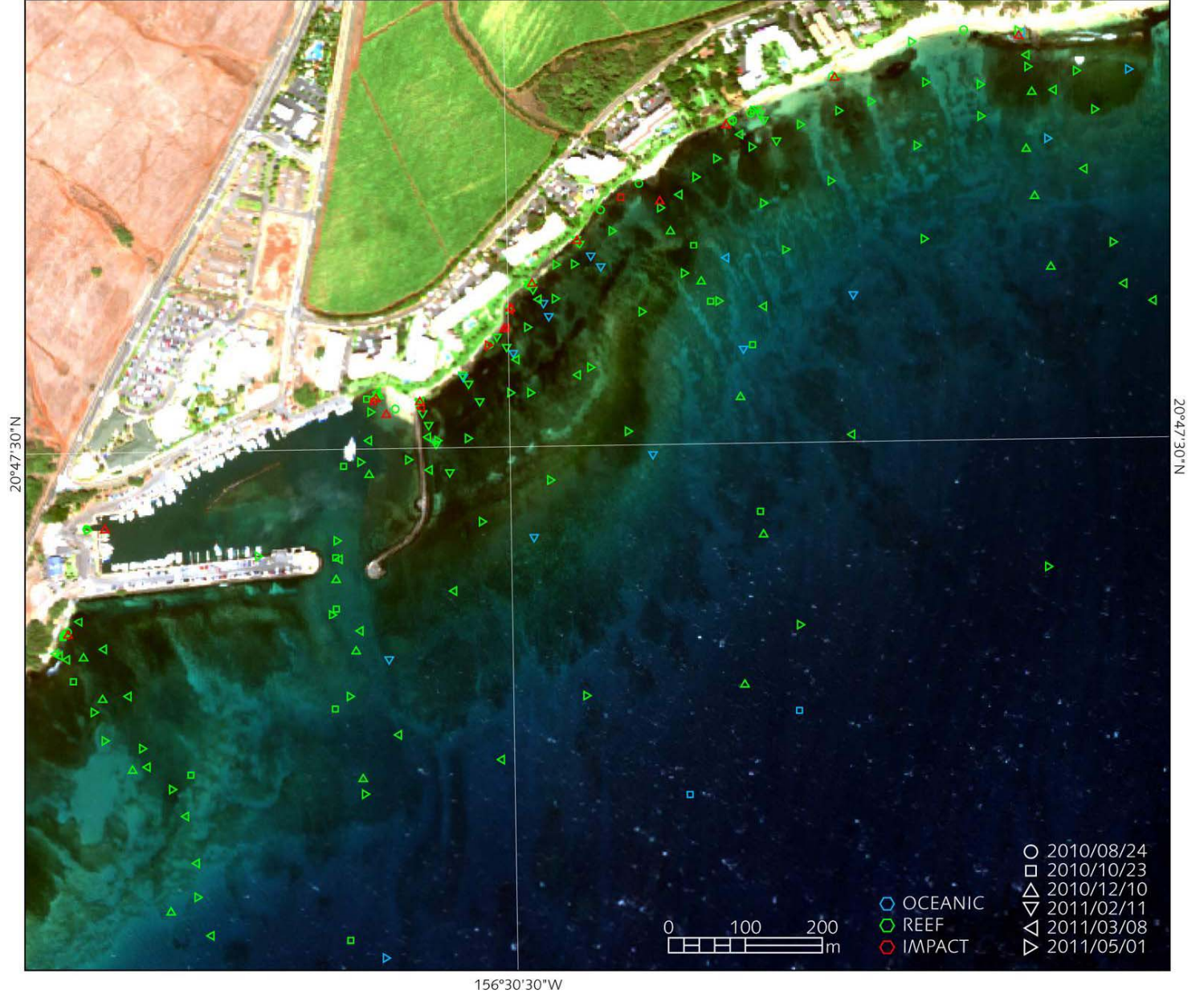
FIGURE 29. Satellite images of Maalaea Bay showing water sampling locations with different symbols representing six sampling days. Color coding corresponds to three “bins” that represent concentrations of \text{NH}_4^+ typically found in the open coastal ocean (blue), typical concentrations found on nearshore coral reefs (green), and “impact” values (red) that represent input from land through groundwater discharge near the shoreline. Top image shows entire study area; bottom images shows area between Maalaea Harbor and Haycraft Beach Park.
