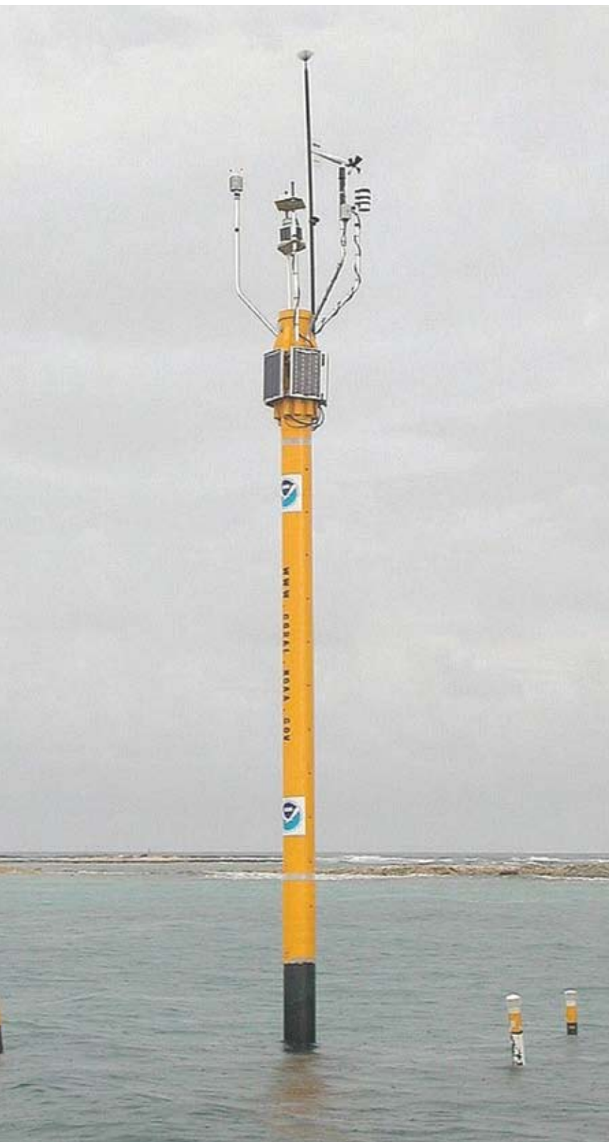
Integrated Coral Observing Network (ICON) Stations are near real-time monitoring stations with an emphasis on data processing for the development of ecological forecasting models. The instruments provide unique in situ information that will aid in improving NOAA's forecasting capabilities (e.g. coral bleaching and climate change).
