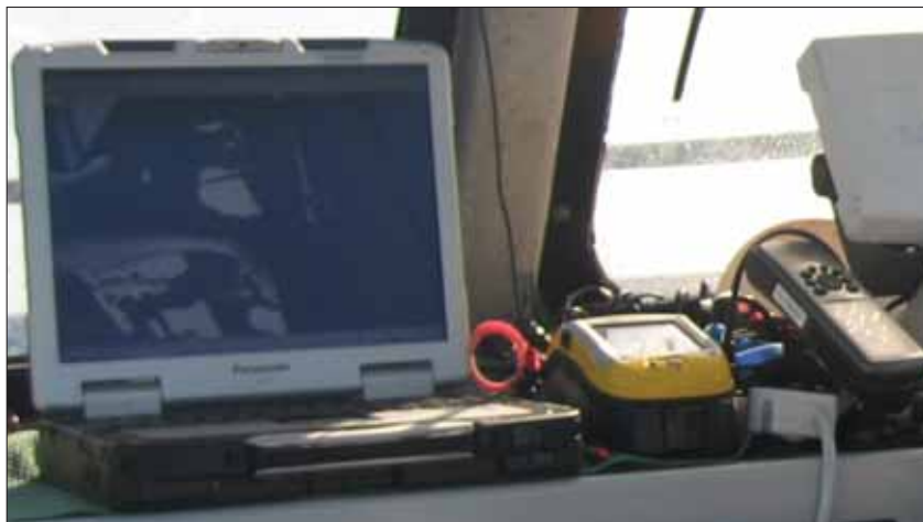
Figure 2.13. The equipment used in the field to collect georeferenced underwater video. The Panasonic Toughbook (left) was used to view the video in real-time. The Trimble GeoXT GPS receiver (middle) was used to record the location of the drop-camera. The Garmin 76 WAAS-enabled GPS unit (right) was used to navigate to each GV site.
