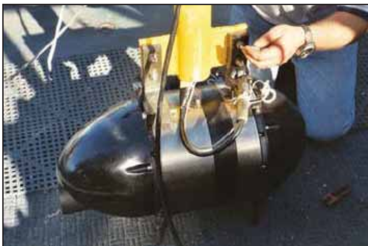
Figure 2.5. The RESON SeaBat 8101 ER (240 kHz) MBES sensor was pole-mounted on the NOAA ship Nancy Foster during two, two week missions in 2004 and 2005. It was used to collect MBES bathymetry and intensity imagery.
