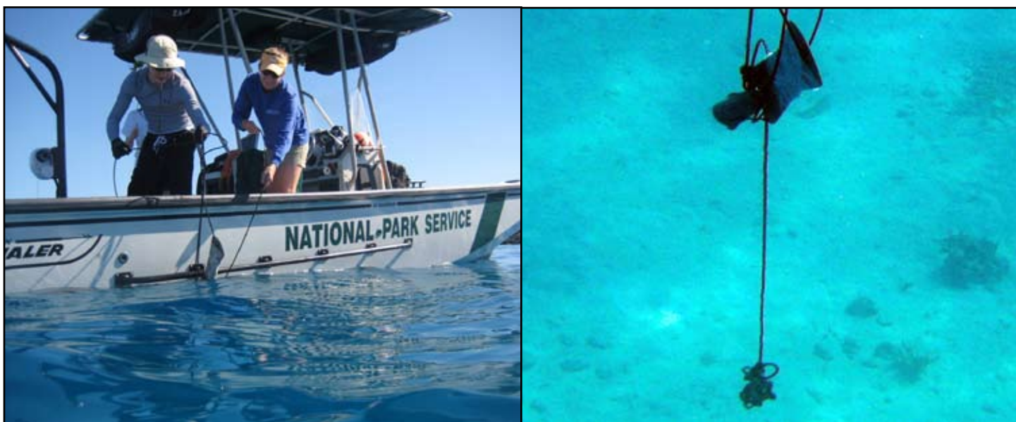
Figure 3.1. Picture of the field crew deploying drop camera (left) and camera approaching bottom (right).
