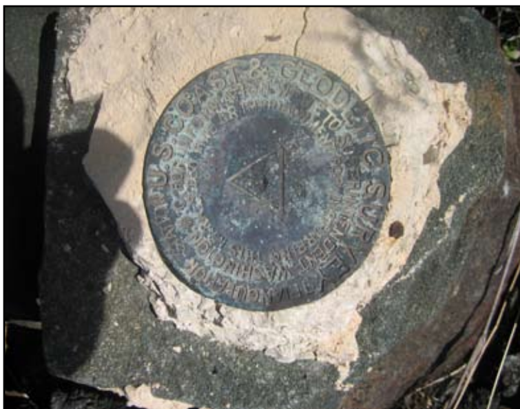
Figure 2.3. Geodetic marker from NOAA's National Geodetic Survey that was used as a ground control point.
