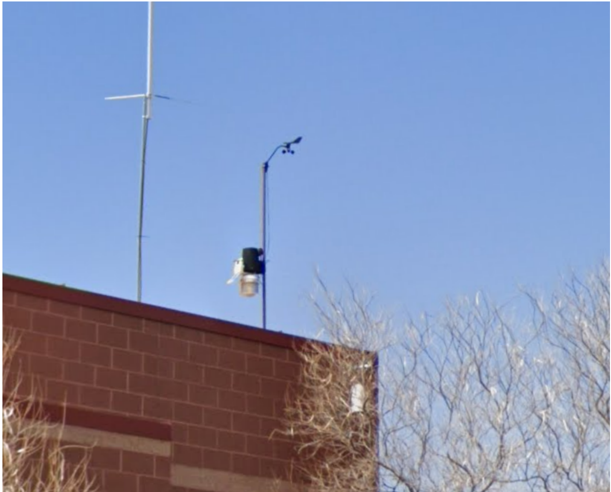
Photograph of the temperature station sited on the roof of the Washington County School District Information Technology building in St. George, UT.
