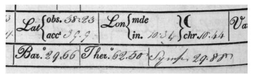
In this example the regular barometric pressure (keyed in F16) is in its normal location, and the 'Symp' pressure is on the right side of the 'Ther' box.
