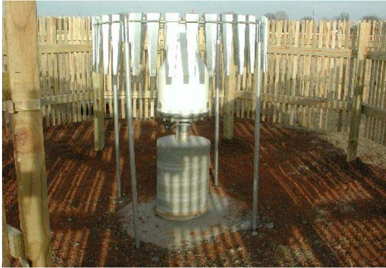
Figure 2. UCSRN rain gauge with single alter and SDFIR wind shields. (From Bruce Baker)
