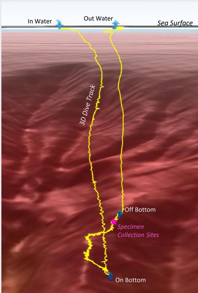
Navigation data that include  $x$ ,  $y$ ,  $z$  values can support 3D displays. ROV *Deep Discoverer*'s 3D dive track, specimen sites, and entry/exit points are displayed above over the 3D tiled bathymetry services.
