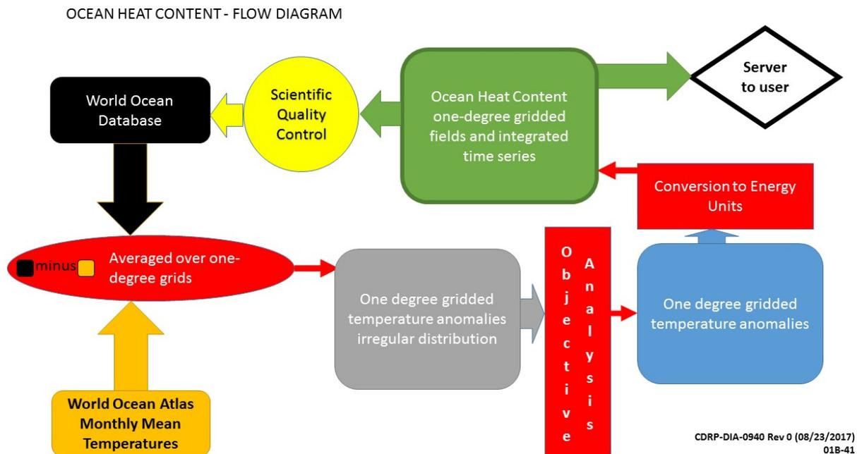
Figure 1: Diagram of OHCA calculation procedure
